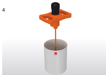
4 Mix resin and hardener thoroughly with stirrer at least 1 minute.
