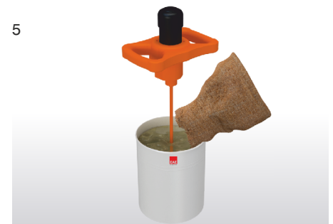
5 Add fillers and mix until homogeneous; at least 5 minutes. Then application must be done within 15 minutes.
